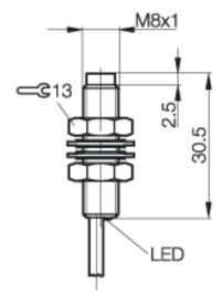
Inductive Sensors BES 516-383-E4-C-PU-03 M8x1 x 30 normally-open Sn=2,5mm unshielded
